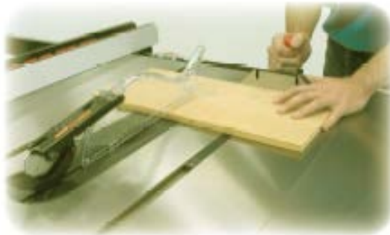
Figure 2 Correct use of miter gauge.
