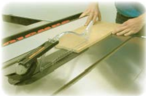
Figure 1 Correct use of rip fence.
